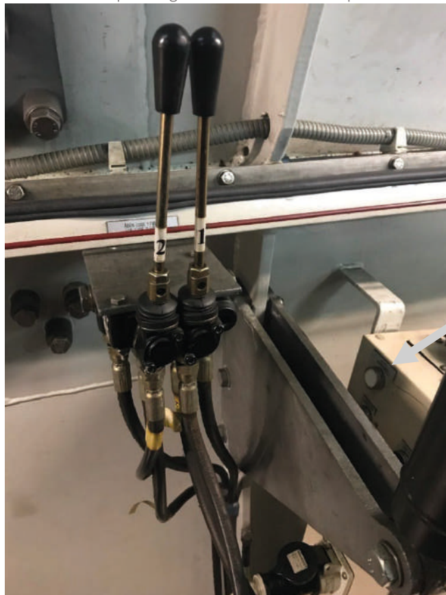
Figure: The handles to be used when opening the two hatches
