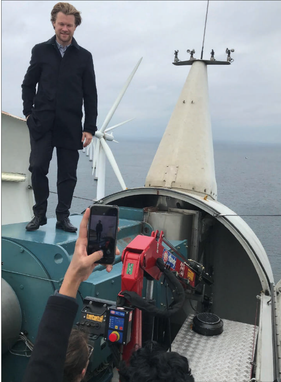
Figure: the emergency stop (red) for the crane can easily be activated just by leaning back without realising it.
